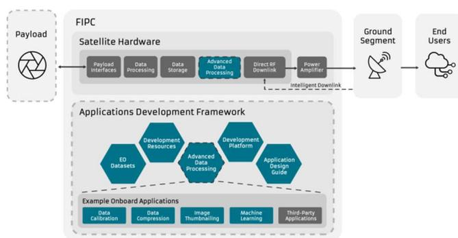
Image 1: Flexible and Intelligent Payload Download Chain for small EO satellites
