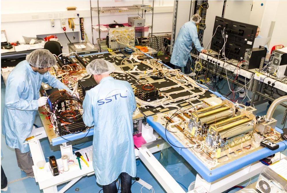
**Galileo FOC payload under manufacture at SSTL**
