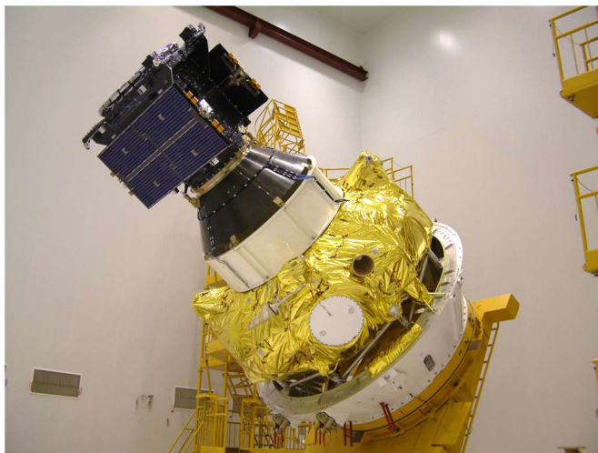
GIOVE-A mounted on the Soyuz Fregate upper stage at Baikonur, ready for launch December 2005. Credit SSTL
