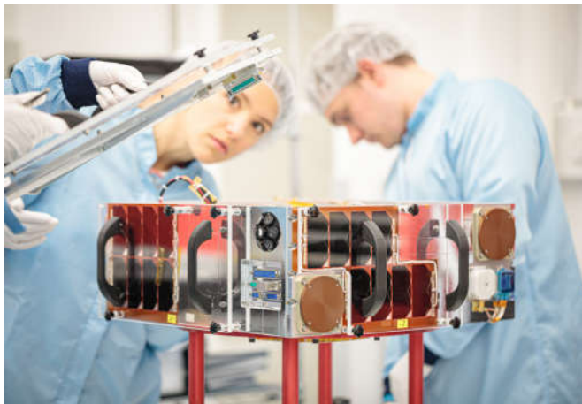
ELSA-d Target satellite during final assembly at SSTL. Credit SSTL/Kathryn Graham
