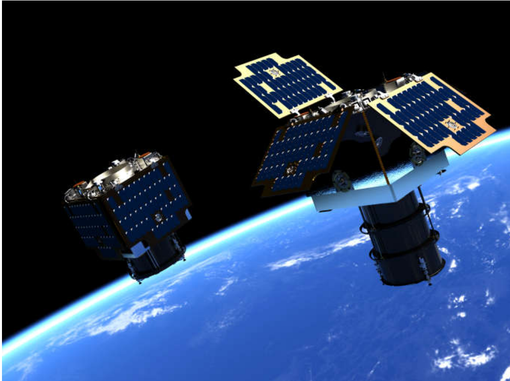
Spacecraft with telescope stowed on the left and deployed on the right. Credit SSTL.
