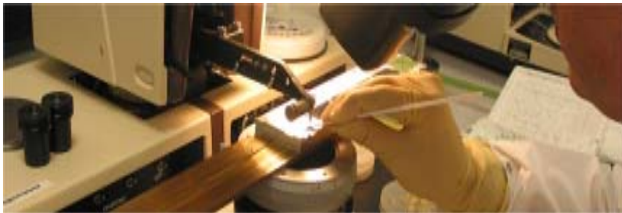
Ultrasonic welding of interconnect to bare cell
