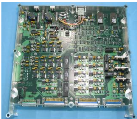
Battery Charge Regulator
