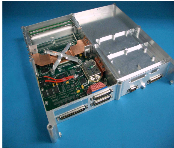
High Speed Solid State Data Recorder and payload data processor
